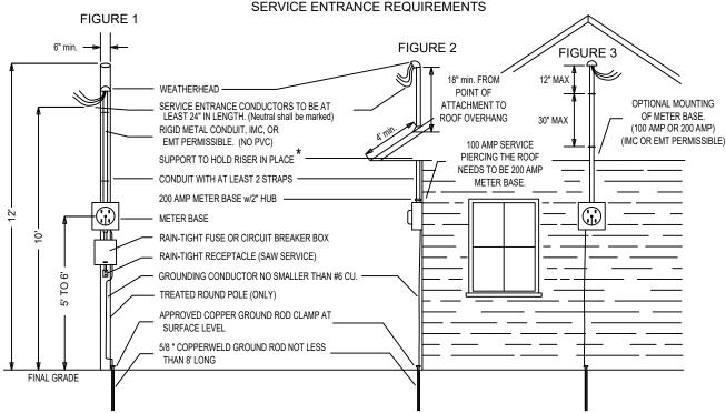
\*NOTE: Where service mast pierces the roof, the roof shall be reinforced with 2"x6" blocking between rafters to provide the necessary support of the service mast, and service mast must be 2 inch rigid metal pipe.
